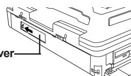
**3** Lift the rear corners, then release the computer from the port replicator.
