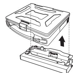
**2** Slide the lever completely to the right side (UNDOCK POSITION) to disconnect the expansion bus connector of the port replicator.
